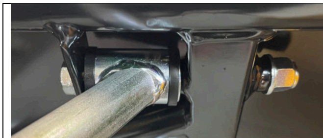
Rear showing white bushings in lower wishbones
