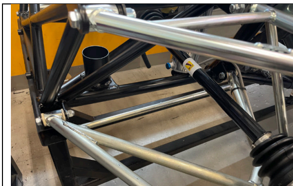
Rear showing white bushings in lower wishbones
