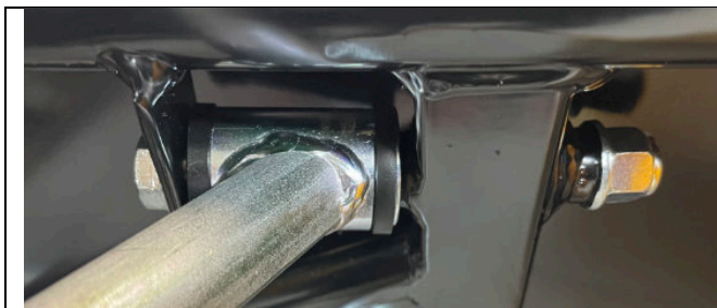
Rear showing white bushings in lower wishbones
