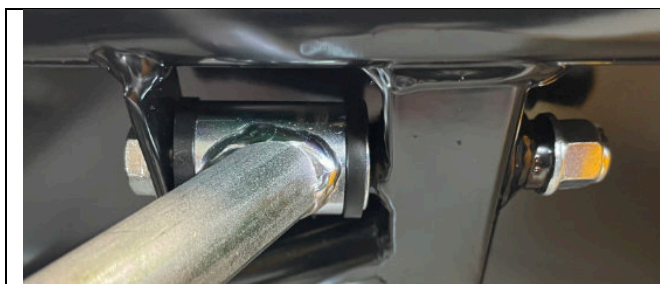
Rear showing white bushings in lower wishbones
